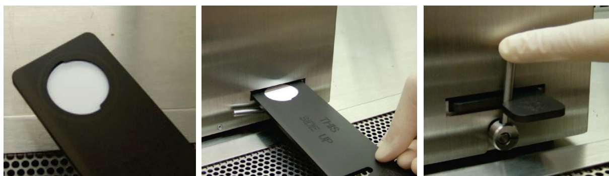
図 3. BIOTRAK Collection Filter Holder and Insertion Process
